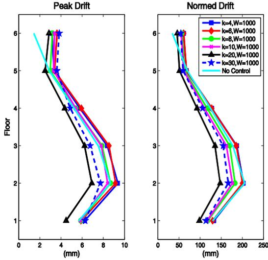
Figure 5 Peak and normed drift by floor due to the El Centro ground motion under MBC as the price to control force conversion factor increases
