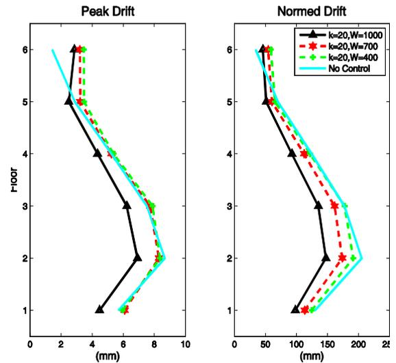
Figure 6 Peak and normed drift by floor due to the El Centro ground motion under MBC as the with diminishing initial wealth allocations
