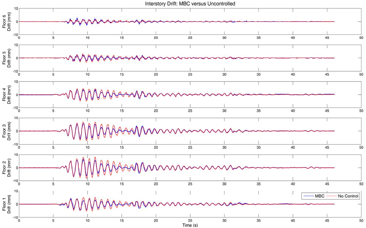
Figure 4 Time-history drift response of the six-story structure to the scaled El Centro ground motion system under MBC ( $K = 20$  and initial wealth  $W_i = 1000$  for all floors)
